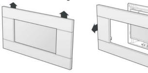
To replace the fascia, line up the four hooks with the matching receptacles on the fire and push the fascia into place and let it drop down, the fascia should now be securely in position
