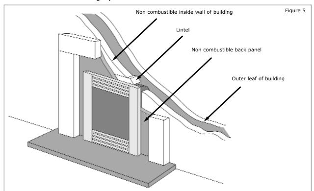
Check the cavity insulation type (if applicable). If cavity insulation is of a loose fill variety, take precautions to prevent excessive loss of material when the inner leaf is opened up by packing the cavity firmly with a minimum 50mm of rockwool or glass fibre. This will hold back any loose material now or in the future.
