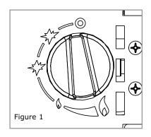
When the pilot lights after one of the two sparks, keep the knob depressed in the nine o'clock position for approximately ten seconds. Now release the knob and the pilot should stay alight. If the pilot is extinguished during use, wait three minutes before repeating the ignition procedure.
