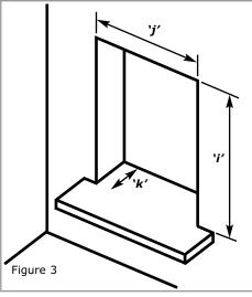
In all installations, the wall or back panel of the installation must be flat, non-combustible and meet the dimensions specified in table 1 and illustrated in figure 2.
