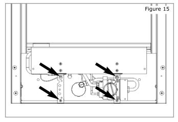
The gas valve is a non-serviceable item. If this needs replacement, remove M15 securing nut holding the valve in place, remove all pipe unions, electrode lead, thermocouple lead and then the complete valve. Replacement must be original manufacturers parts. Re-assembly is the reverse of removal. Ensure operating pressures are as stated in Section 2; Appliance Data.
