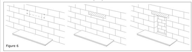
The hearth may now be put in place (If fitted). Again this should not bridge the cavity where it projects into the wall space. Finally install the fireplace or fire surround and back panel/marble to its finished location.
