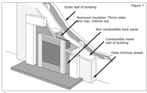
Installation as per method 2 (recessing into a wall)
