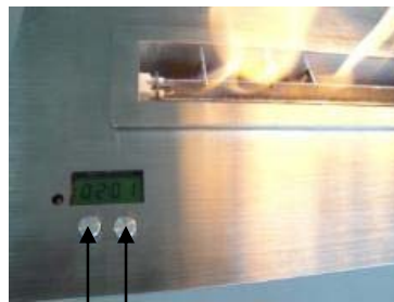
tank opening 2 1 on/off switch
